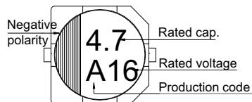
$\phi D = 4 \sim 6.3 \text{ mm}$
