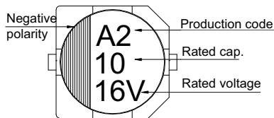
$\phi D = 8 \sim 10 \text{ mm}$
